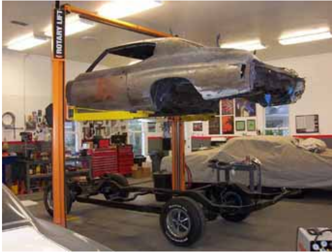
Fig. "A" shown is a full rise two-post surface lift from Rotary Lift used by MCC member Mike Martin of Madison.
